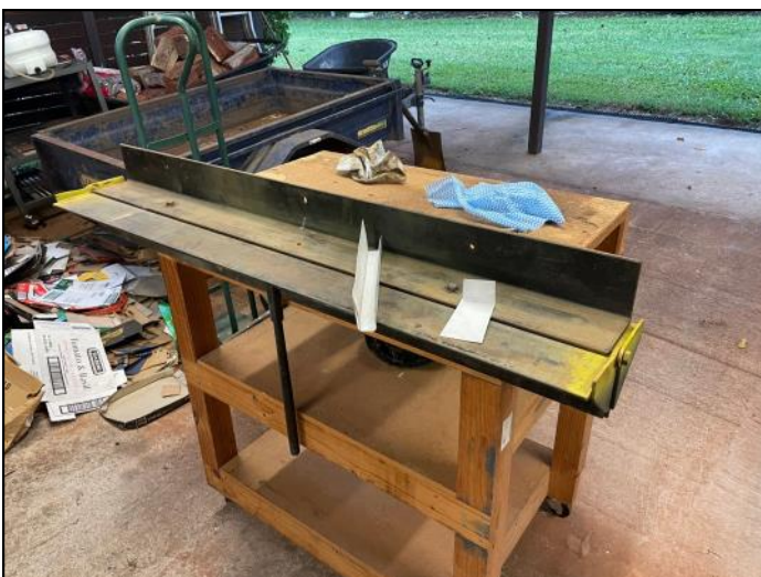
Using a break to bend the aluminium panels. First time I have used one and it works very well
