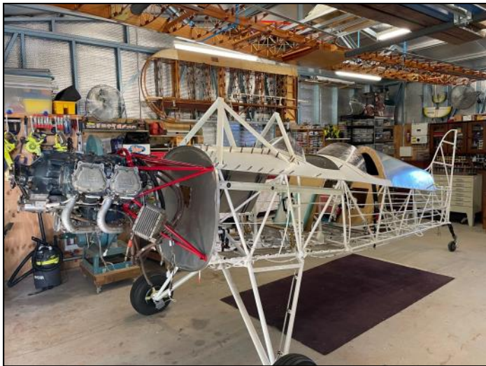
Engine temporarily attached to help plan for engine control cabling, and electrical and plumbing components on the firewall.
