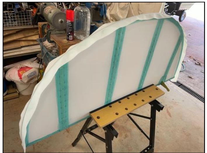
Edge tape being heat-shrunk around the edge of the rudder. Time consuming but comes up nicely.
