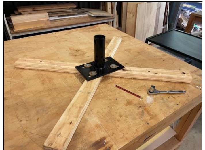
Making the rotisserie for the fuselage. Modified a standard engine stand.
