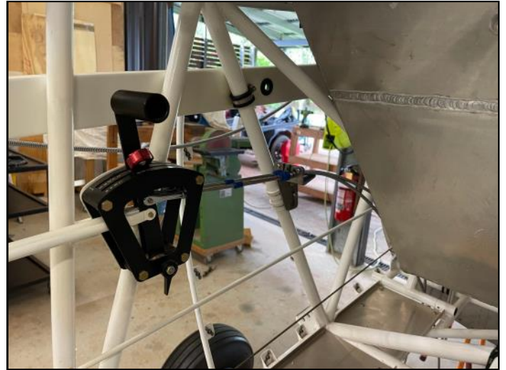
Showing the throttle and mixture connections to the front (pax) cockpit.
