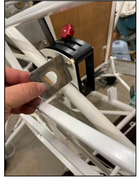
New prop control bracket for the rear cockpit. Nice and close to the throttle.
