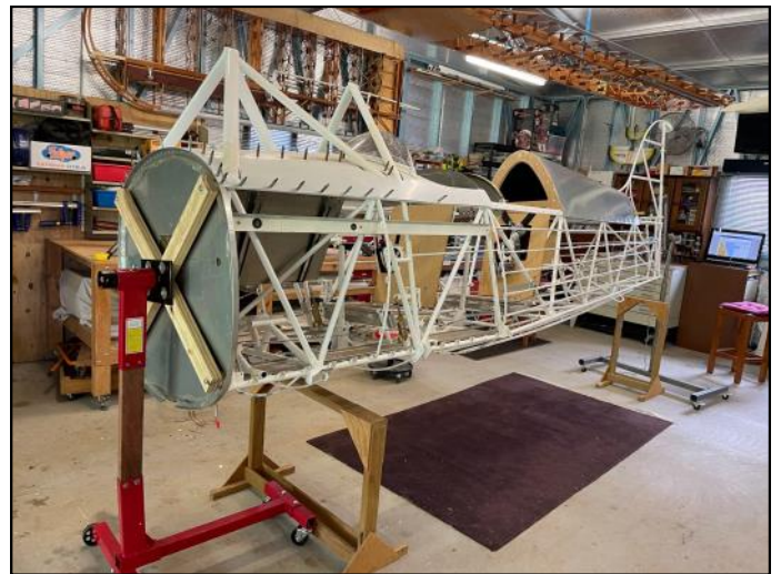
Fuselage mounted on rotisserie. I made the rear rotisserie stand previously (see a previous post).
