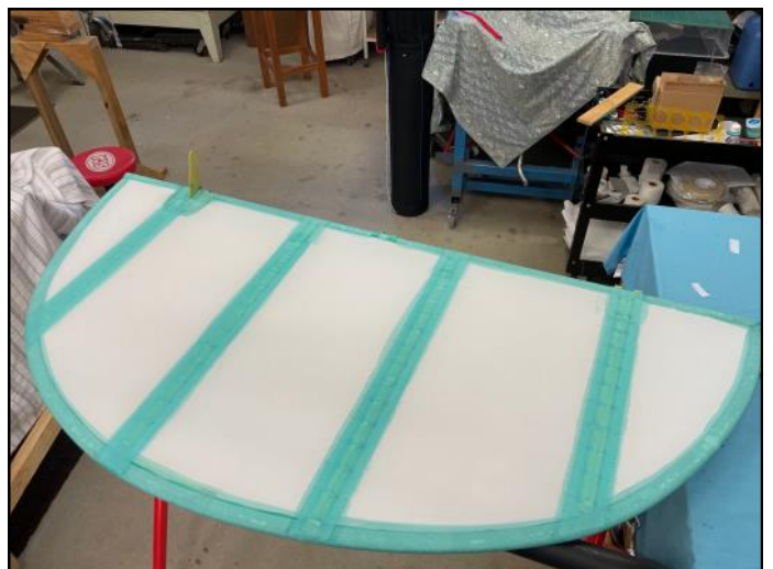
Tapes glued over the stitching for a nice smooth transition over the stitches.
