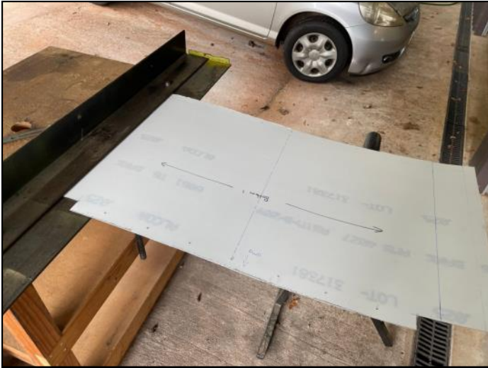
Bending the lip of the bottom panel to form up the side.
