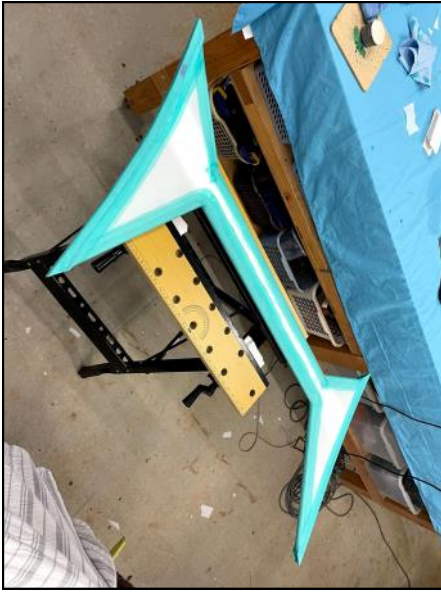
Interplane struts covered - now that was an interesting job!
