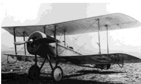
Bristol D Scout powered by an 80HP Le Rhone rotary
