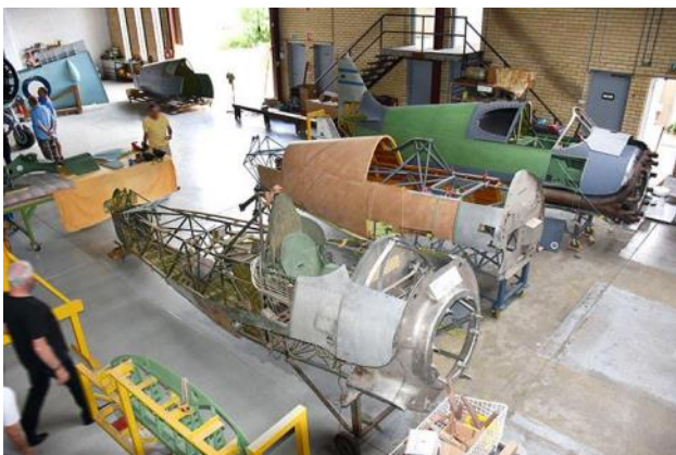
CAC CA-12 Boomerang A46-77, A46-92 & A46-55 fuselages on show with A46-54 nearing completion
