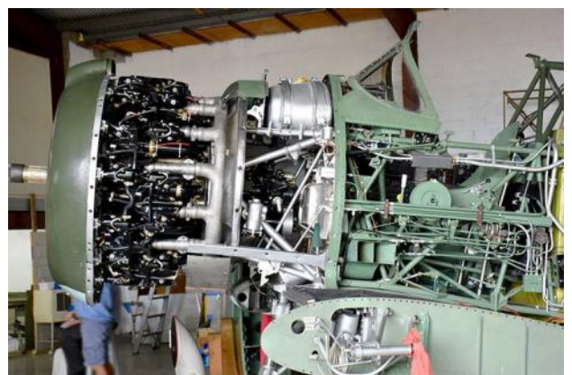
CAC CA-12 Boomerang A46-54 with Pratt & Whitney R-1830-90 Twin Wasp 14 Cylinder radial engine of 1,200 hp (895 kW) - what a beauty!
